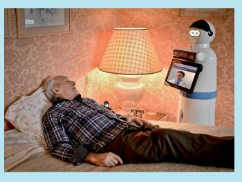
**KOMPAI** can securely transfer information to certified health platforms relying on its system of sensors. It can also manage follow-up surveys using a vocal system, and centralize all connected e-Health objects.
